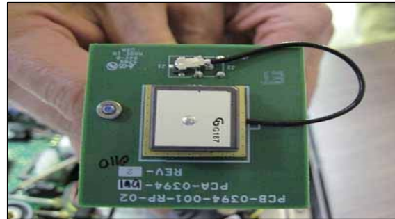
ACTIVE GPS ANTENNA CABLE ROUTING (PASS)
