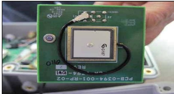
ACTIVE GPS ANTENNA CABLE ROUTING (FAIL)
