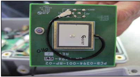
ACTIVE GPS ANTENNA CABLE ROUTING (FAIL)
