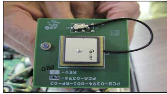
ACTIVE GPS ANTENNA CABLE ROUTING (PASS)
