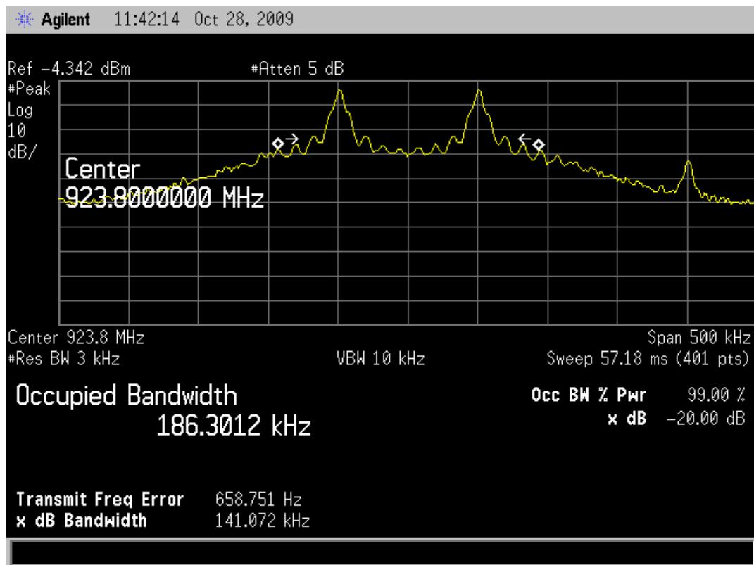
**RSS-Gen 7.2.3 (RSS-GEN 4.10)****Receiver Spurious Emission Limits****7.2.3.2 Radiated Measurement**
