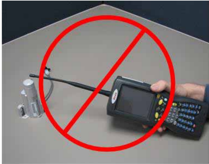
Figure 13: Wrong Position for Handheld
