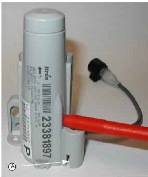
Figure 11: Magnet Placement for Programming Mode
