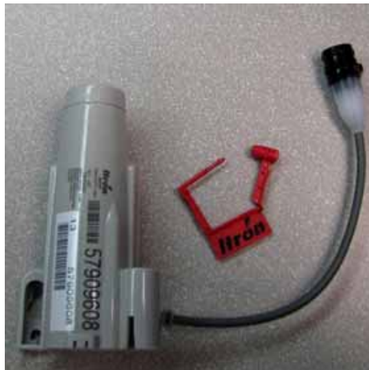
Figure 1: 60WP Endpoint with Inline Connector and Tamper Seal
