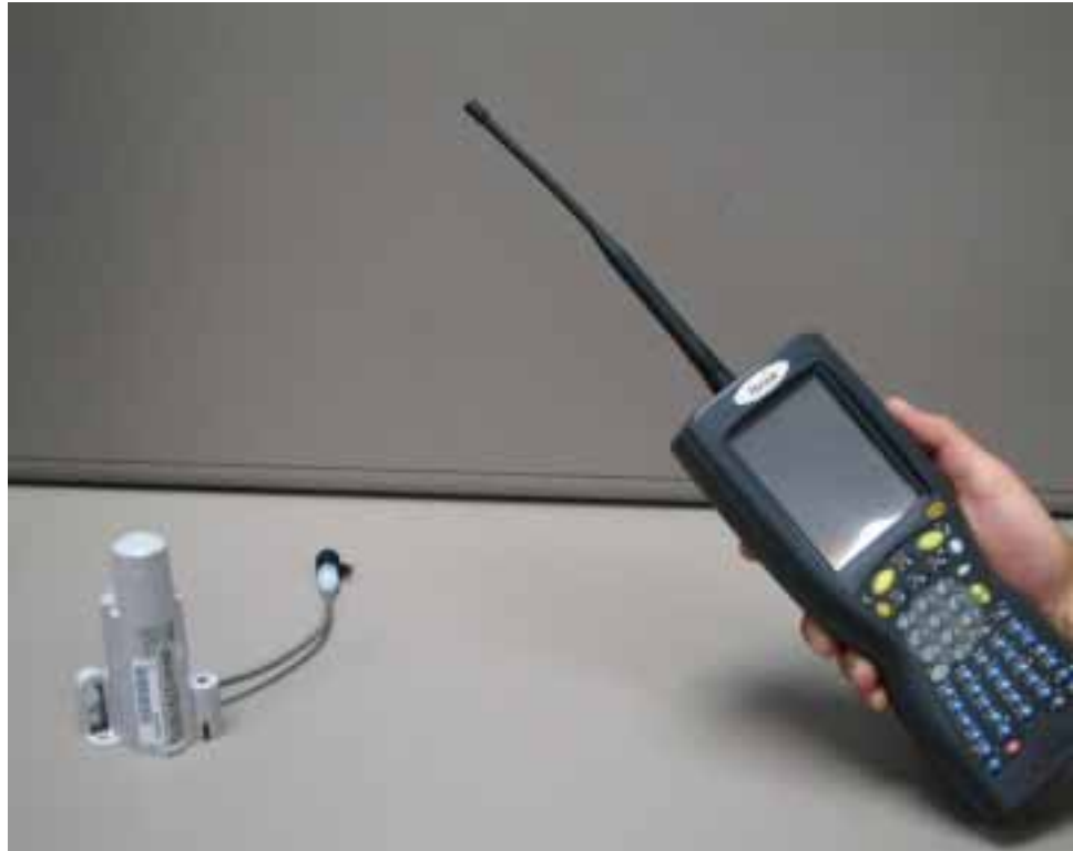
Figure 12: Programming the 60WP - Correct Position for Handheld Antenna
