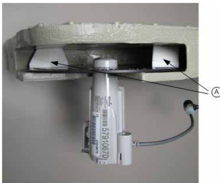
Figure 6: Correct Position With Foam Spacers on Each Side of Slot
