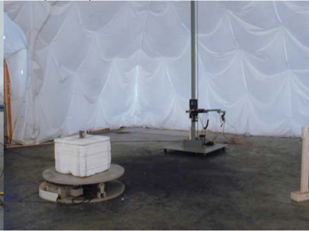
Setup for measurement of the Tx fundamental without pre amplifier
