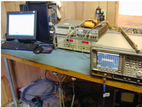
EMC analyzer with the Antenna correction Factor, Amplifier Gain, and Coax loss programmed into internal tables.
