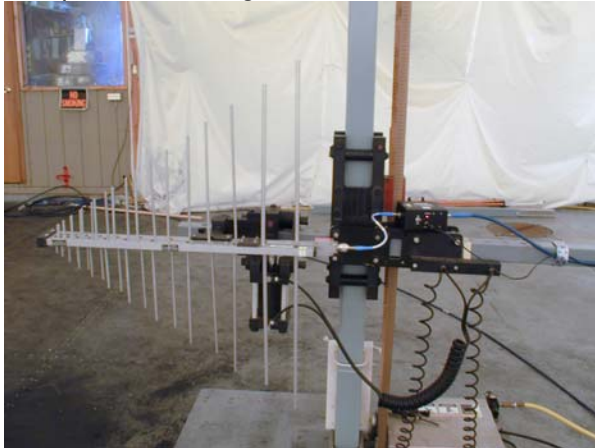
Setup for measuring the receiver radiated emissions
