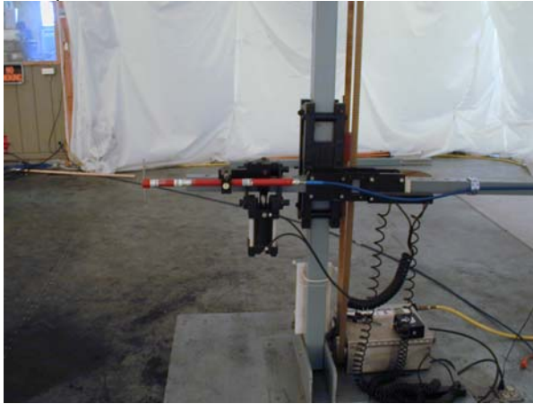
Setup for measuring the receiver radiated emissions
