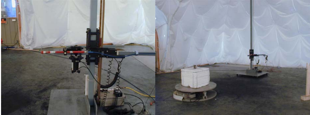
Setup for measuring the receiver radiated emissions
