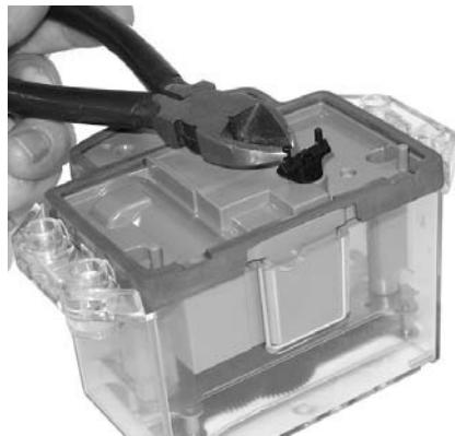
2. Set the wriggler to the desired position for mounting the ERT module assembly to the meter.
