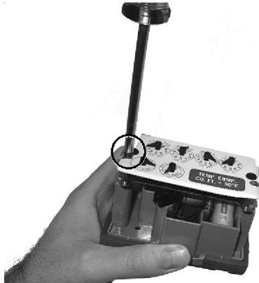
10. Tighten the right-hand index mounting screw.
