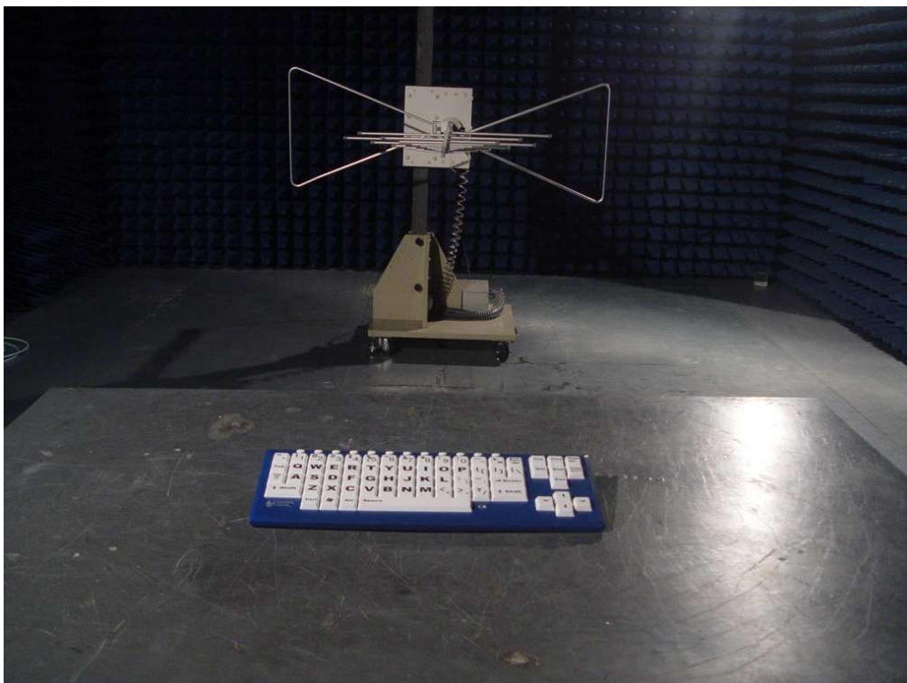
Photograph 2: Set-up for Spurious Emissions (30MHz-1GHz)
