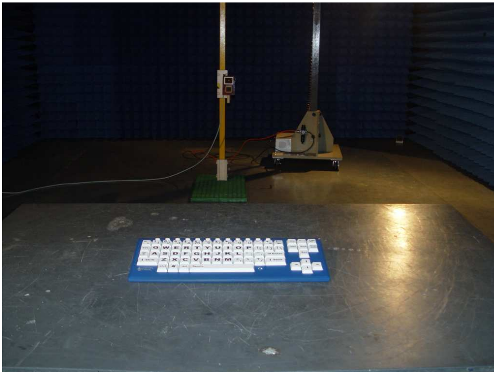
Photograph 4: Set-up for Spurious Emissions (18GHz-26GHz)
