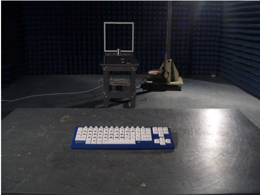
Photograph 2: Set-up for Spurious Emissions (30MHz-1GHz)
