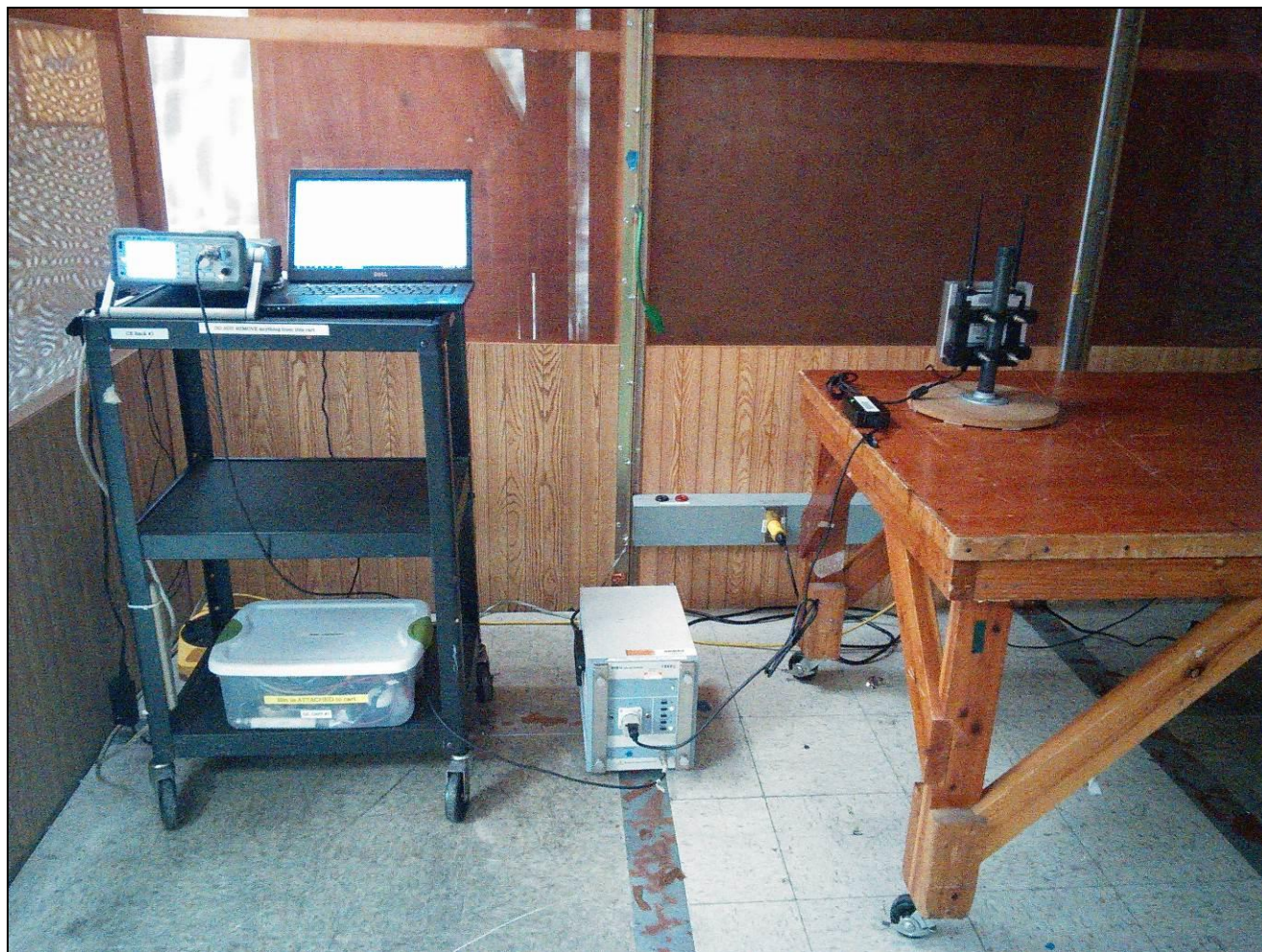
Photograph 4. Conducted Emissions, 15.207(a), Test Setup
