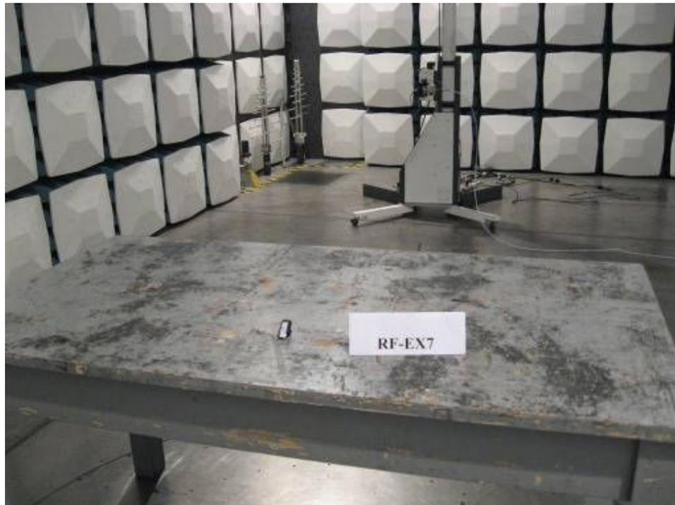
**Photograph 5: Set-up for Radiated Emissions**
