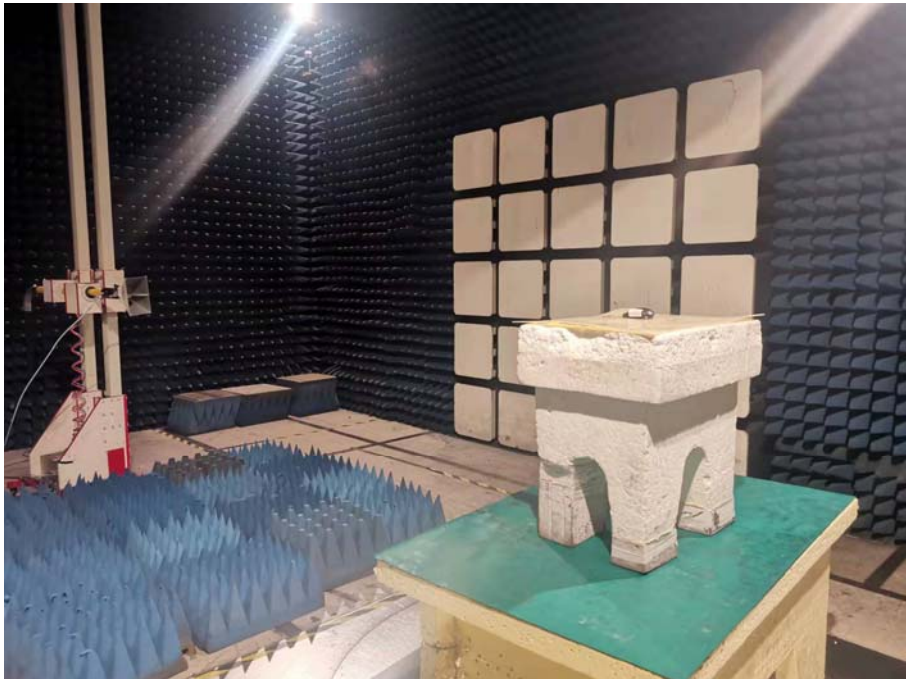
Spurious Emission Test Setup (Above 1GHz)
