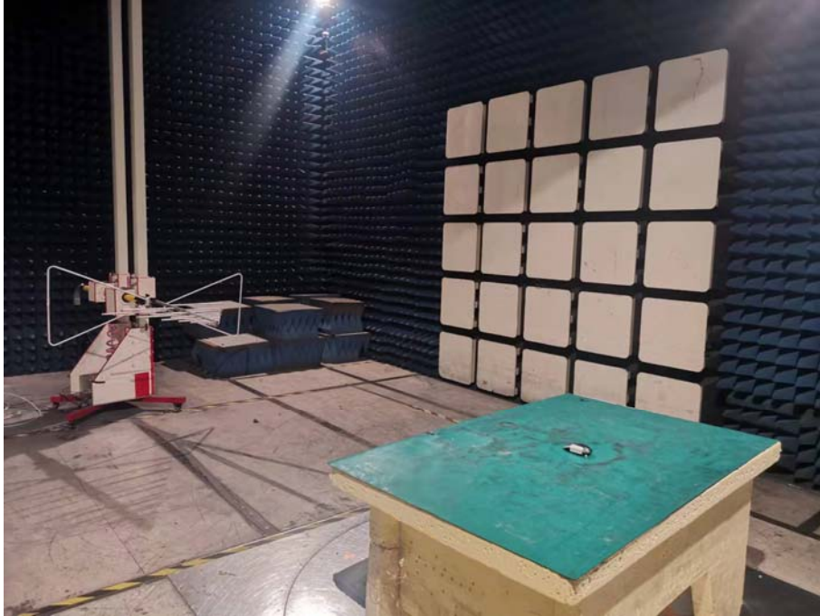
Spurious Emission Test Setup (Above 1GHz)
