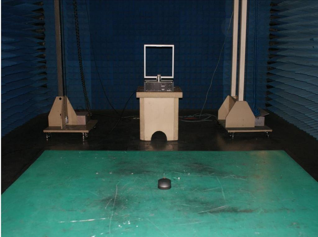
Photograph 2: Set-up for Spurious Emissions of 30MHz – 1GHz
