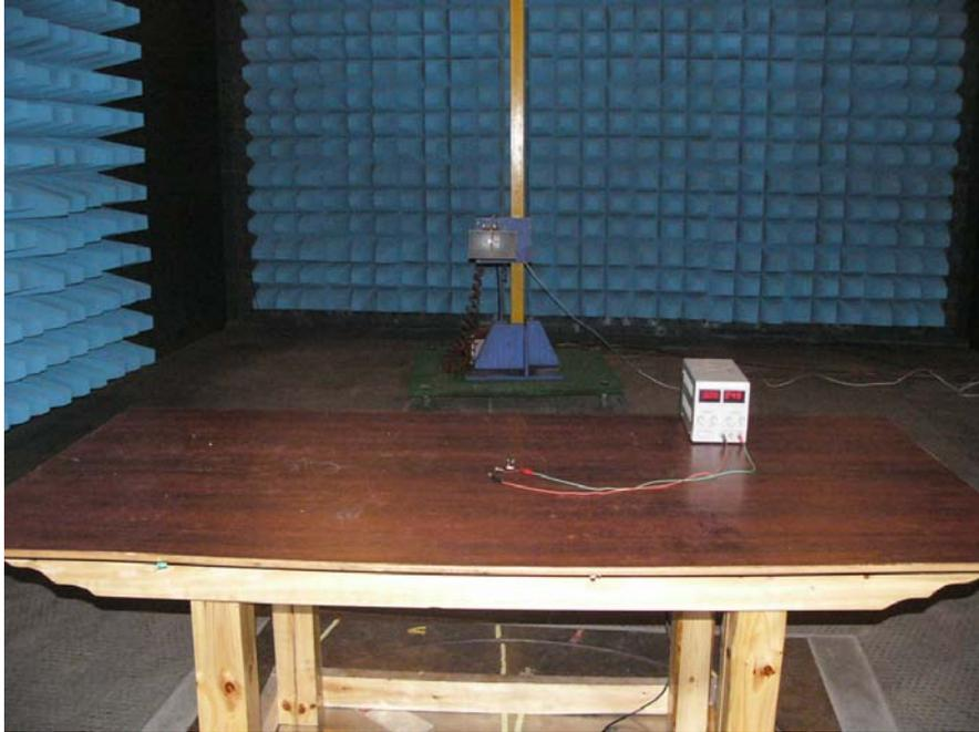
**Power Line Conducted Emissions Setup Photos**
