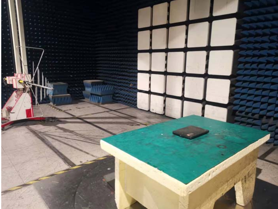
Spurious Emission Test Setup (Above 1GHz)
