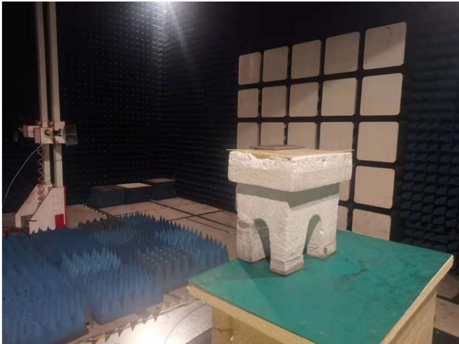
Spurious Emission Test Setup (Above 1GHz)
