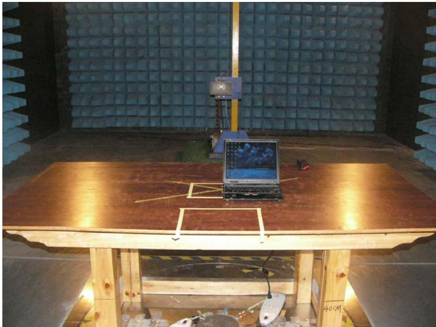
**Power Line Conducted Emissions Setup Photos**
