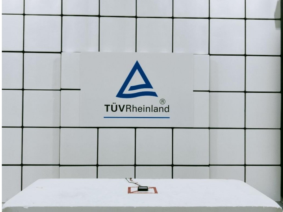
Photograph 1: Test Setup for Spurious Emissions (Front View 1)
