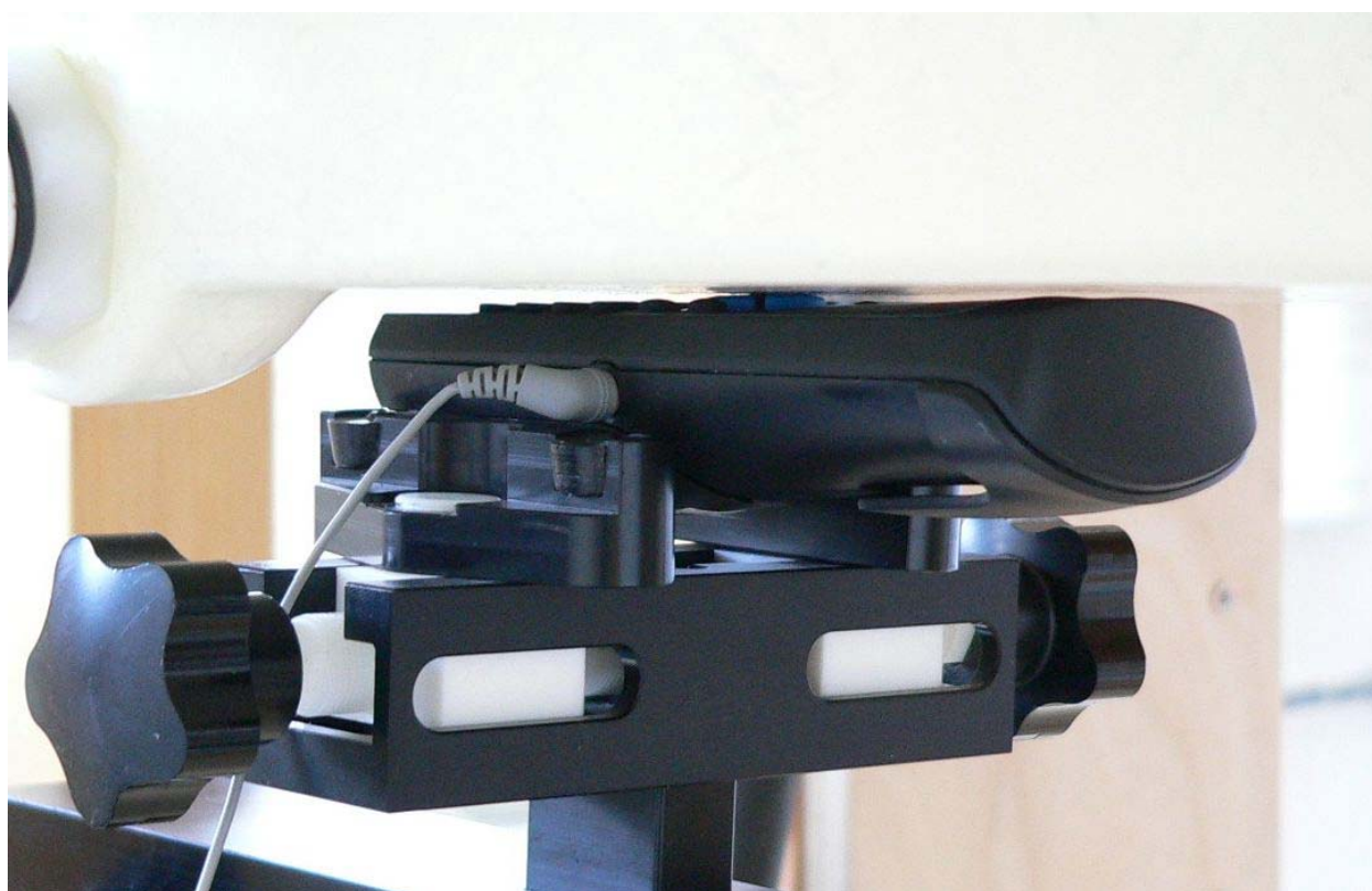
Fig. 23: Body worn, position 4 with no-name headset, display towards the phantom.
