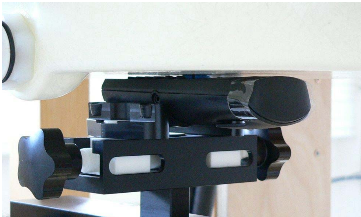
Fig. 22: Body worn, position 3 without accessory, display towards the phantom.
