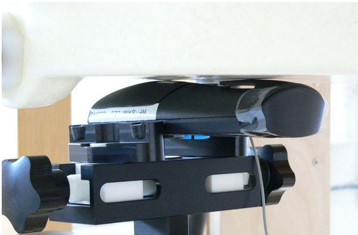
Fig. 21: Body worn, position 2 with no-name headset, display towards the ground.
