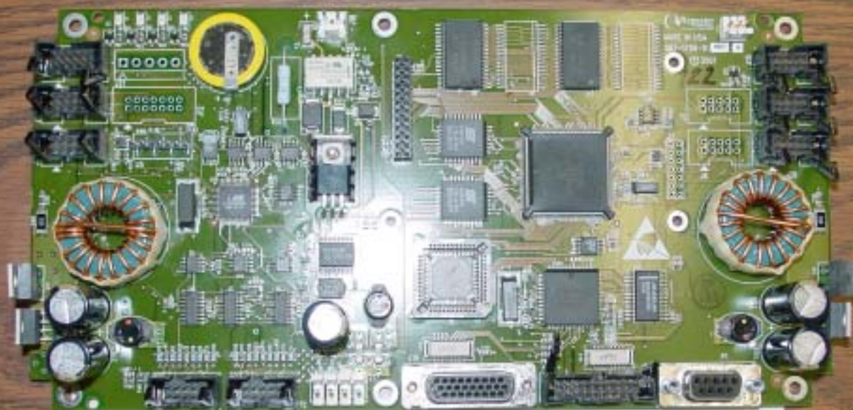
087-1706-01 Alarm Control Unit (Front)
