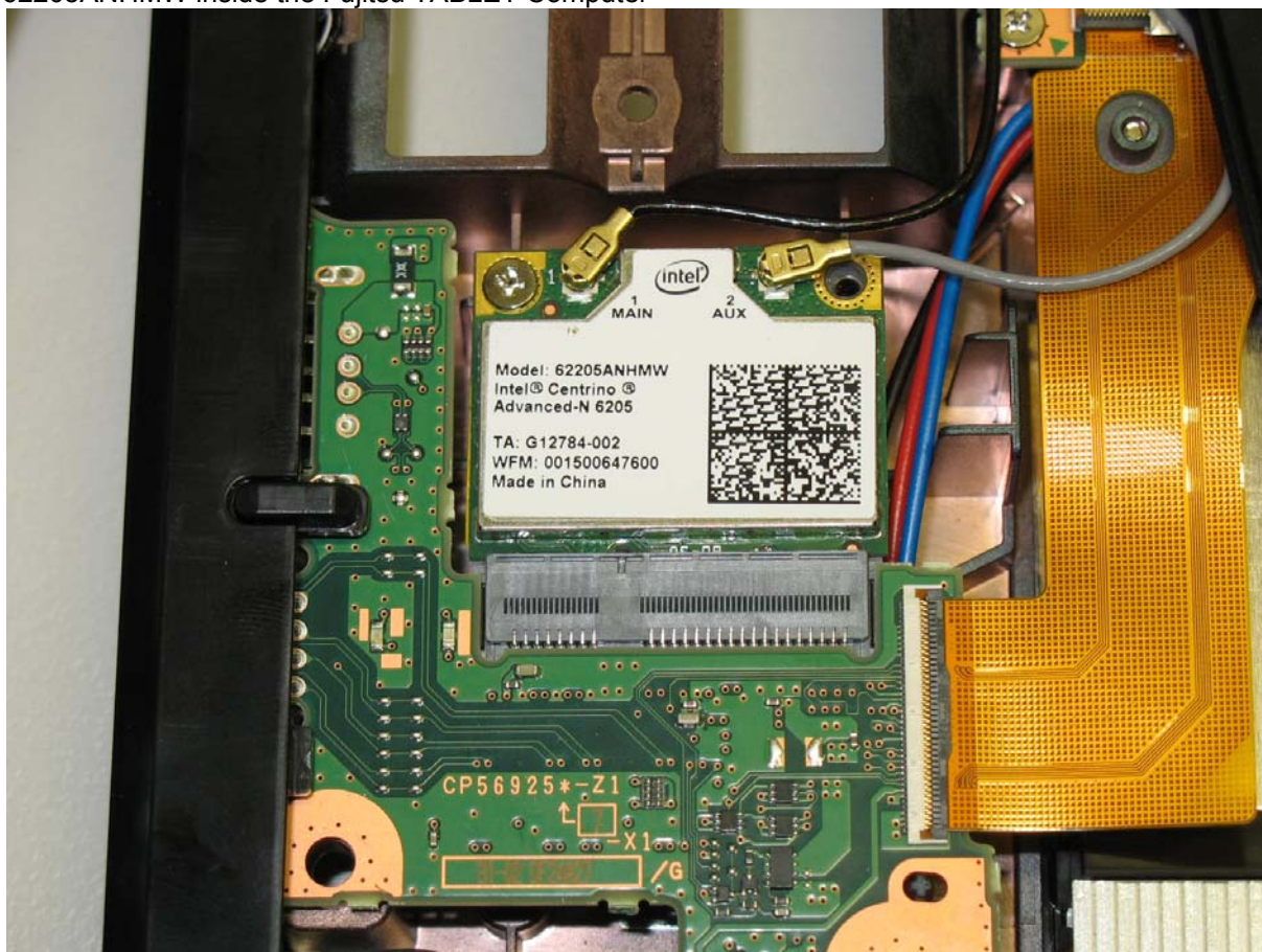
62205ANHMW inside the Fujitsu TABLET Computer
