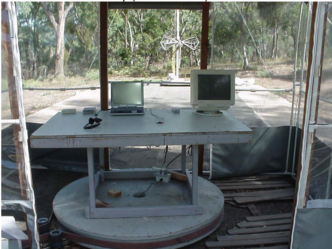
Radiated Emissions Test Setup (10 metre distance)
