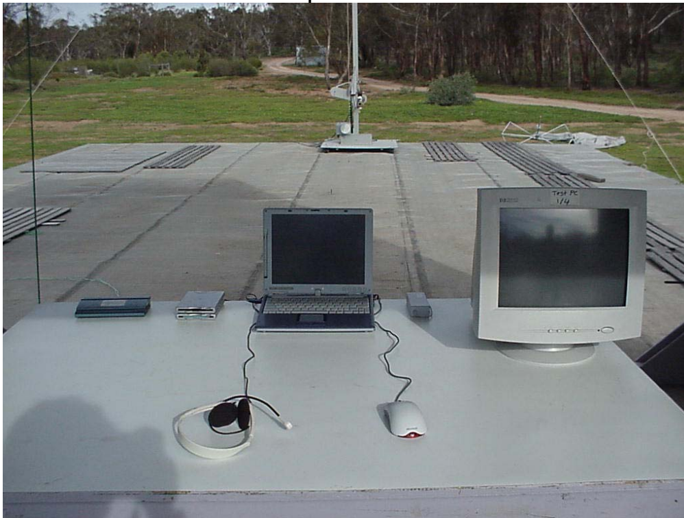
Radiated Emissions Test Set Up – 30 to1000 MHz
