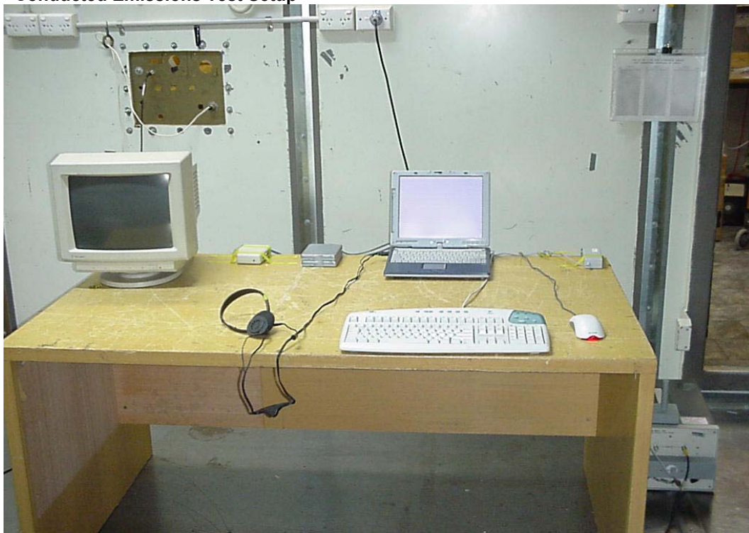
Conducted Emissions Test Setup
