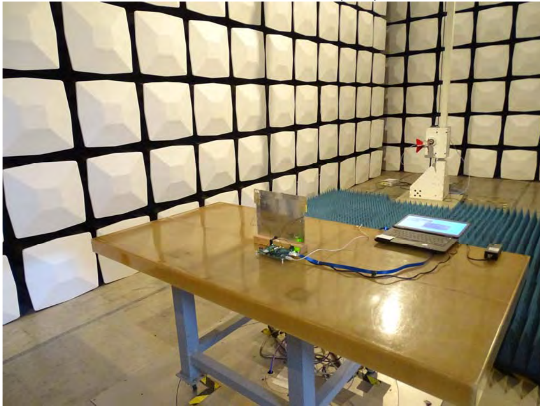
Back View of Radiated Test (Horn)
