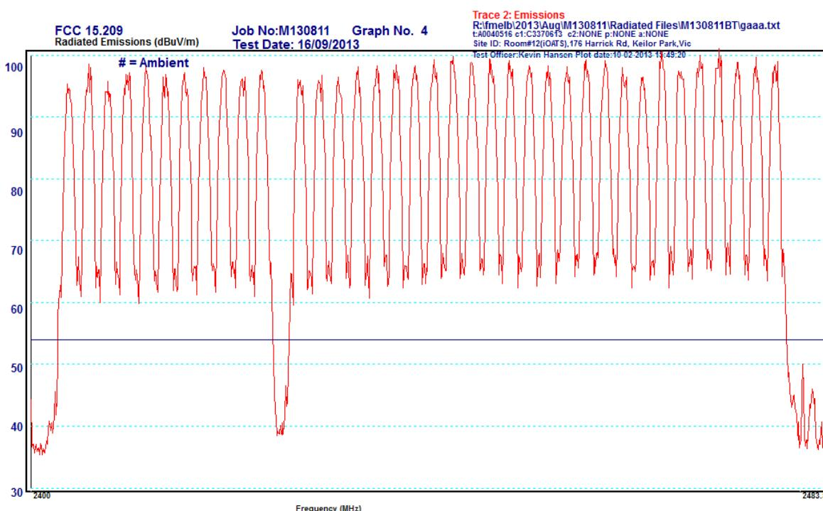
No emissions using the peak or average detectors exceeded the 2310MHz to 2390MHz and 2483.5MHz to 2500MHz restricted band limits.
