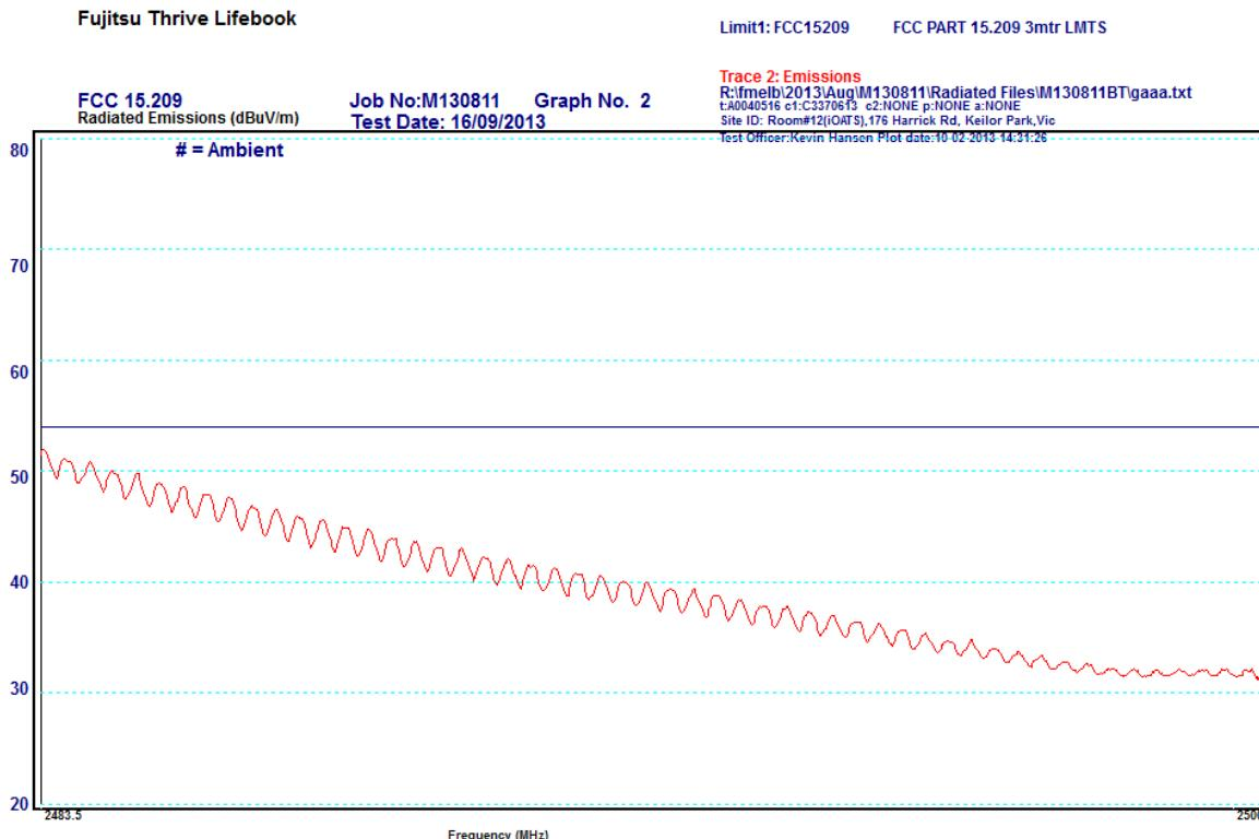
**Result:** No emissions using either peak or average detector exceeded the 15.209 limits in these bands.
