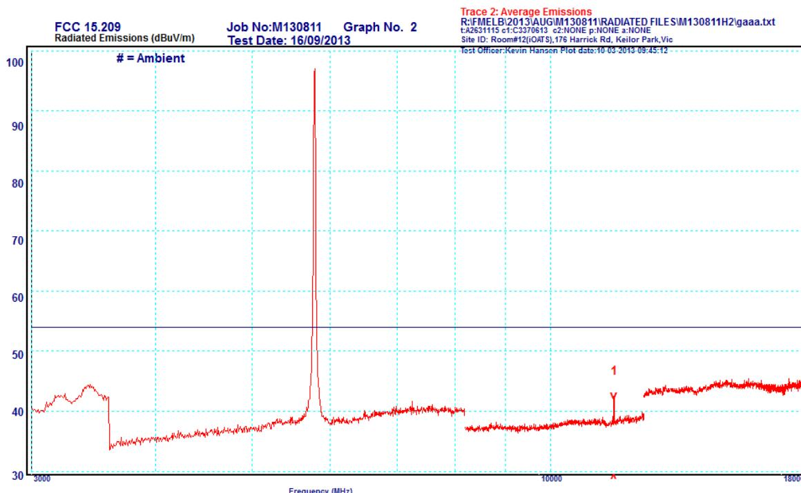
**Result:** Harmonics and spurious emissions were recorded up to 40 GHz. Other emissions were confirmed low with both RBW and VBW reduced. The worst case emissions complied with the FCC limits of sections 15.209 and 15.247.
