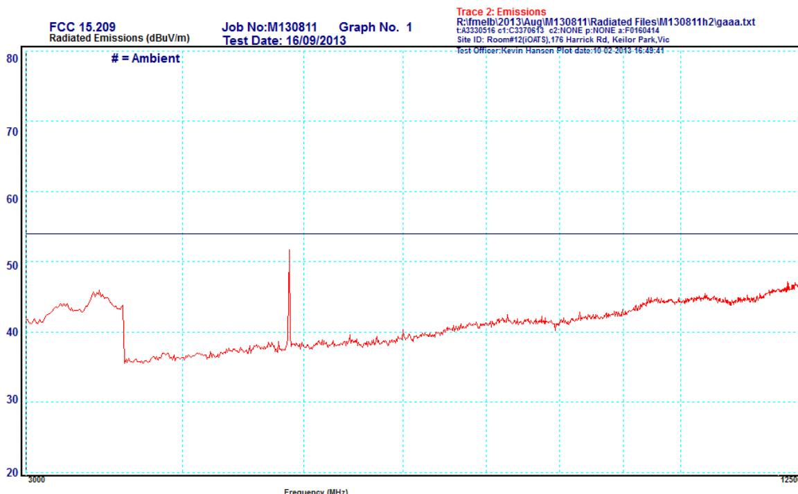
**Result:** Harmonics and spurious emissions were recorded up to 25 GHz. Other emissions were confirmed low with both RBW and VBW reduced. The worst case emissions complied with the FCC limits of sections 15.209 and 15.247.
