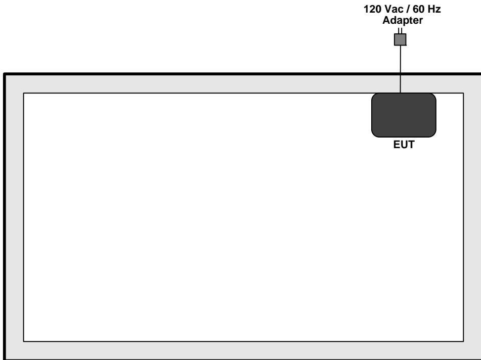
**For radiated emissions 30MHz~1GHz**
