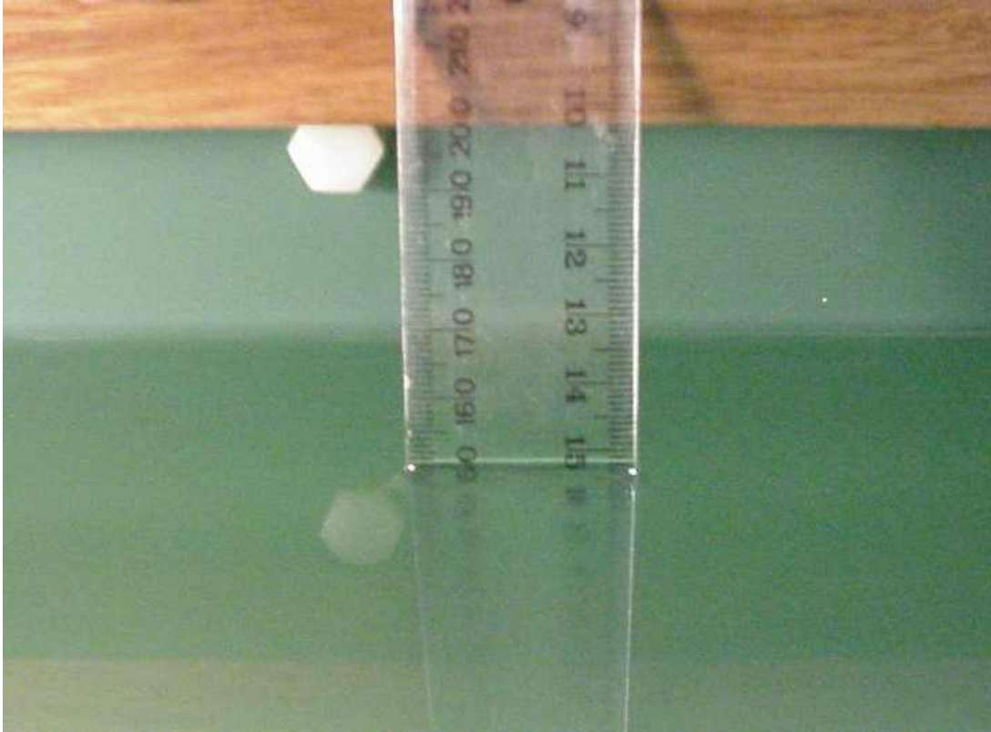
Photo of liquid Depth in Flat Phantom
