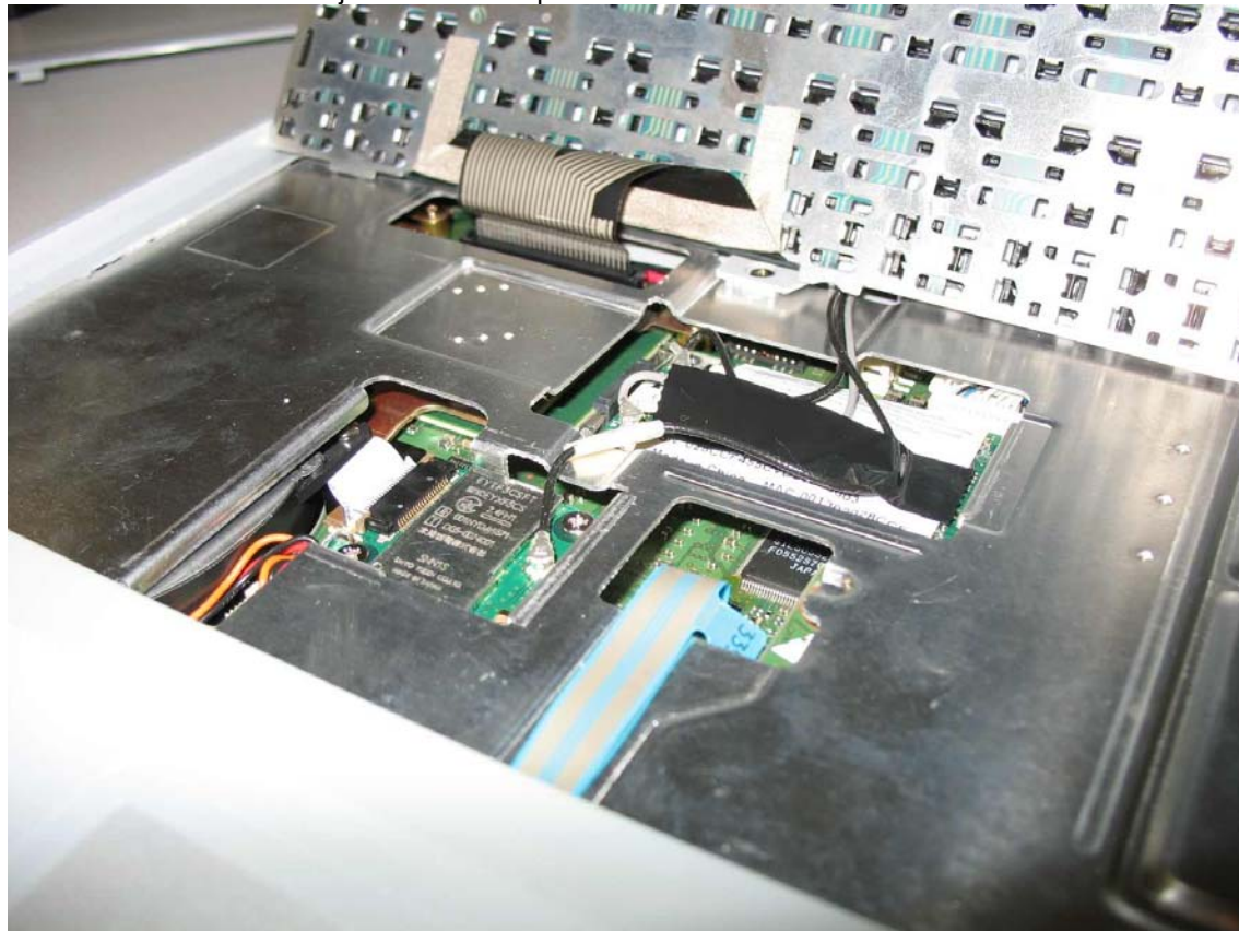
WM3945ABG inside the Fujitsu Tablet Computer
