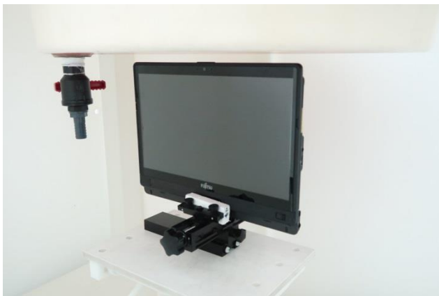
Edge1, Test Separation 14 mm
