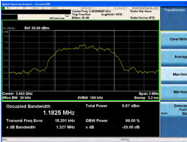
20dB Bandwidth plot on channel 39 (3Mbps)
