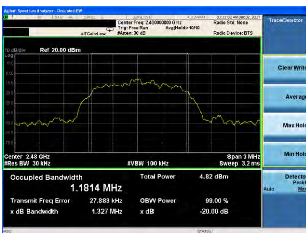
20dB Bandwidth plot on channel 78 (3Mbps)
