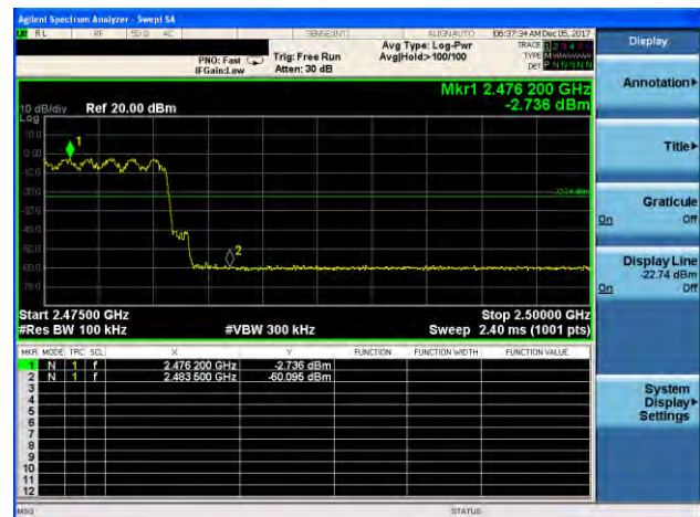
8-DPSK: Band Edge-High Channel (Hopping Mode)
