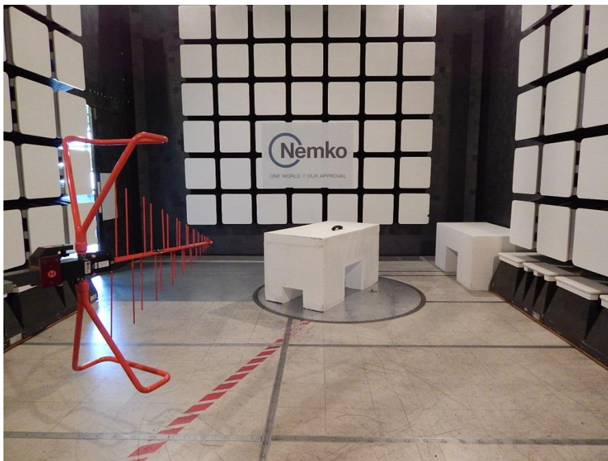
Figure 8.5-69: Radiated spurious (out-of-band) emissions setup photo – 30 to 1000 MHz
