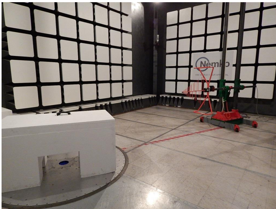
Figure 8.5-70: Radiated spurious (out-of-band) emissions setup photo – 30 to 1000 MHz
