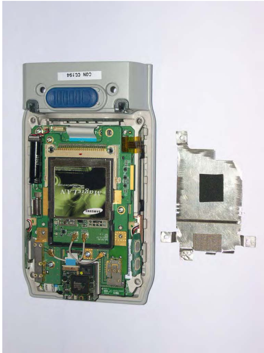
CN30 Console with 2610CF Shield Removed
