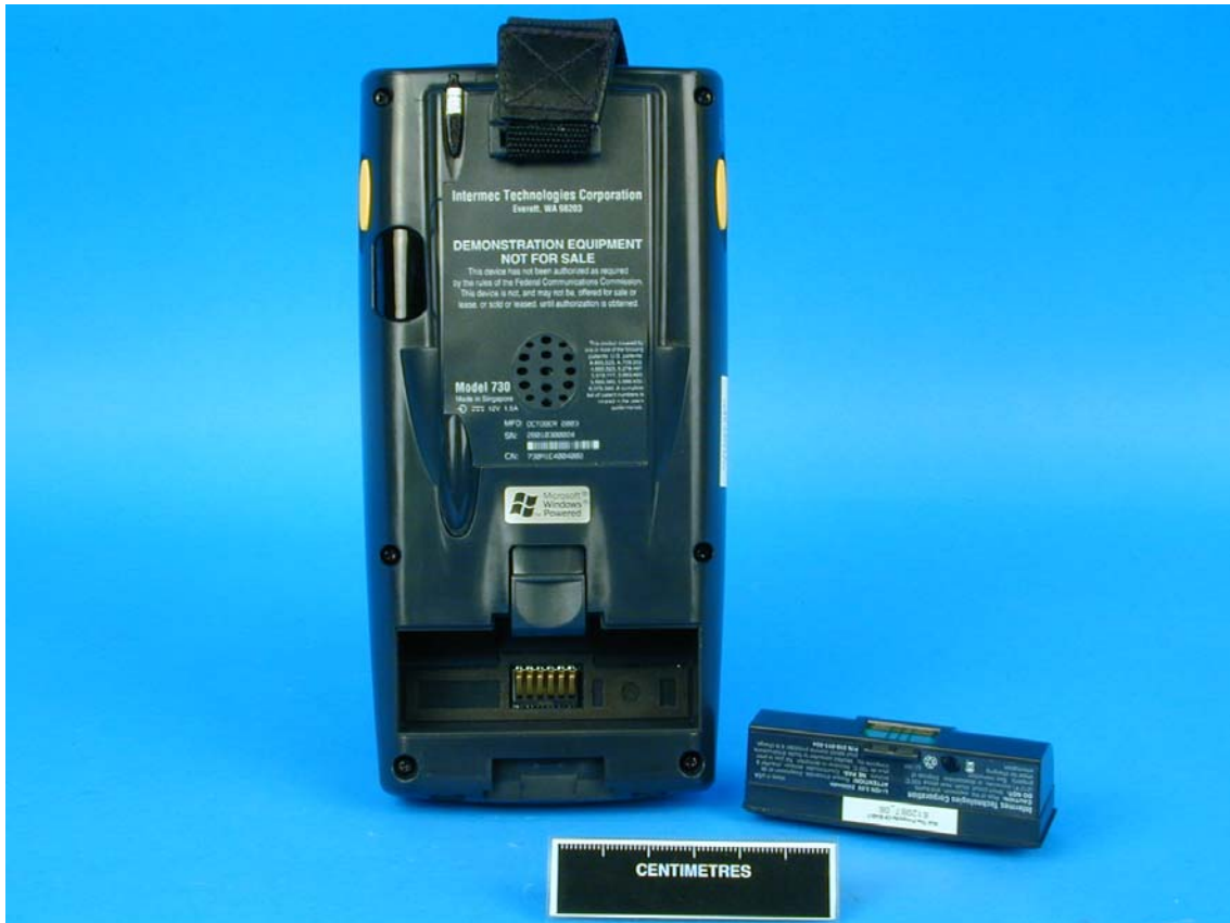
Figure 24. Rear View of the Intermec 730 Handheld Computer, with the battery removed.
