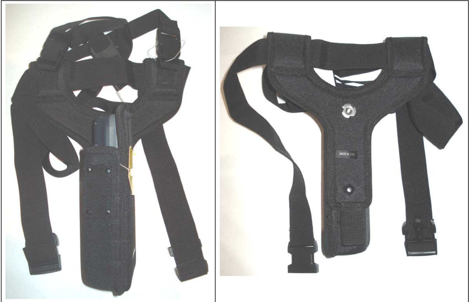
DUT with Holster & Y-Belt Body-worn accessory – Left Side of DUT facing user's body (antenna side closest to user)
