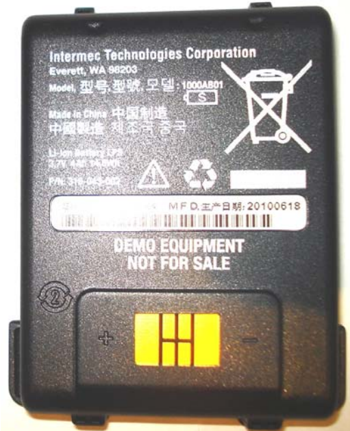
DUT Lithium-ion Battery (Model: 1000AB01)
