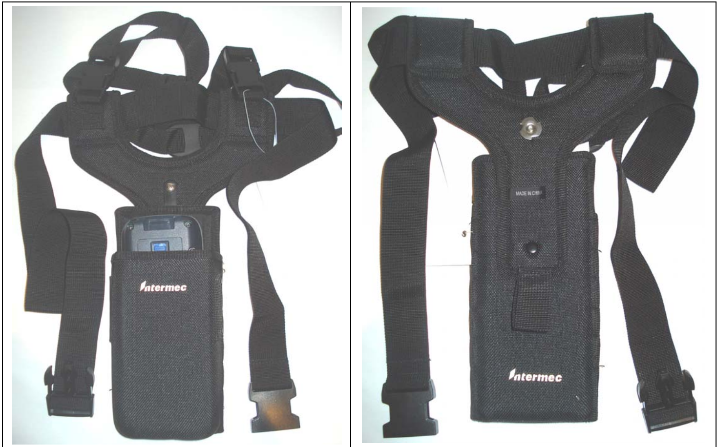
DUT with Holster & Y-Belt Body-worn accessory – Front Keypad Side of DUT facing user's body
