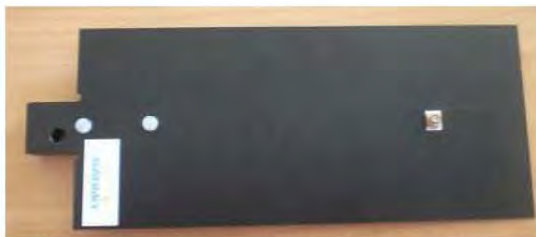
Figure 1 – Satimo COMOHAC Validation Dipole
