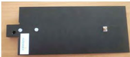
Figure 1 – Satimo COMOHAC Validation Dipole
