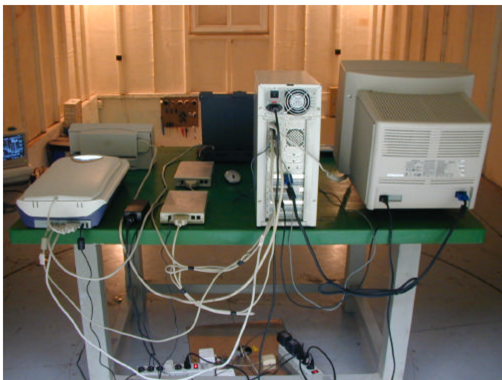
Back View of Radiated Test (Mode 4—Link PC, W/TMA, W/1394 Cable (1.5m)+ FAIRWAY VE50-150A (Adapter))
