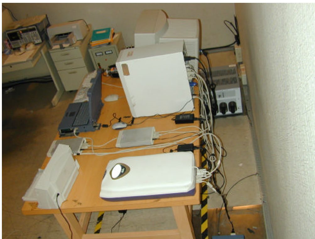
Back View of Conducted Test (Mode 3—Link PC, W/TMA, W/USB Cable (1.5m)+LI-SHIN LSE9802B1540 (Adapter))
