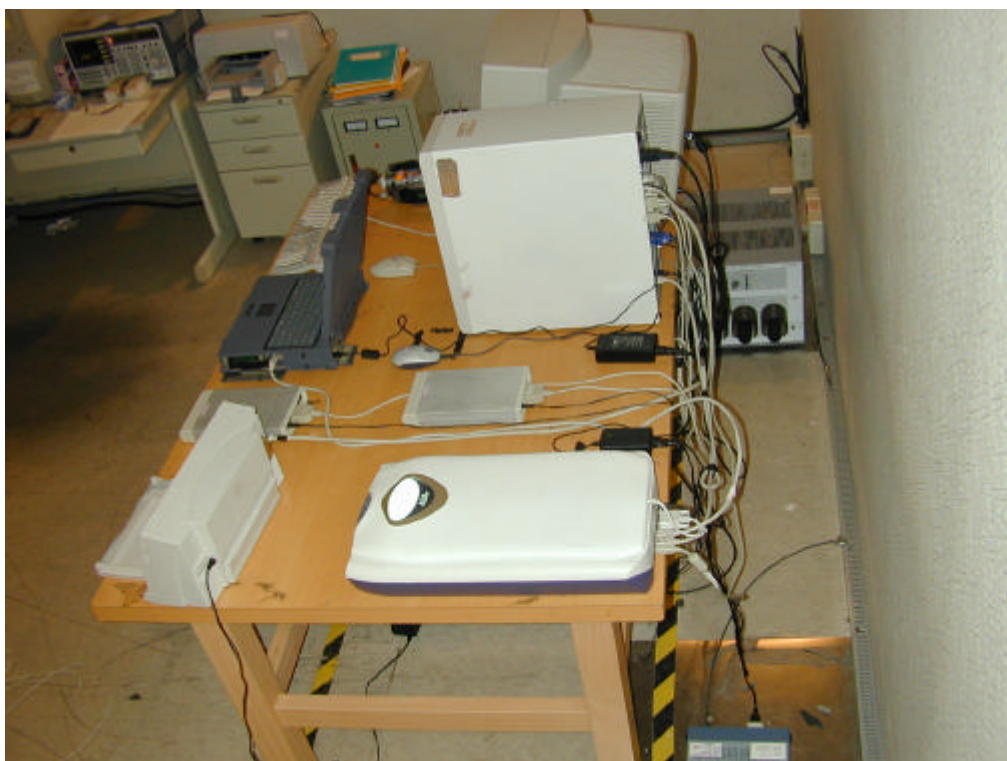
Back View of Conducted Test (Mode 2—Link PC, W/TMA, W/1394 Cable (1.5m)+LI-SHIN LSE9802B1540 (Adapter))
