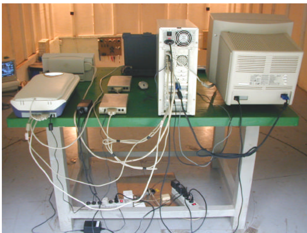
Back View of Radiated Test (Mode 1—Link PC, W/TMA, W/USB Cable (1.5m)+ FAIRWAY VE50-150A (Adapter))
