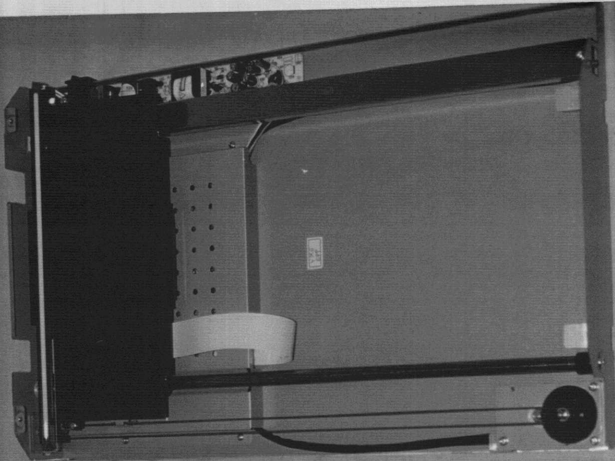
Figure 6 Top Cover Removed, Frame of Internal
