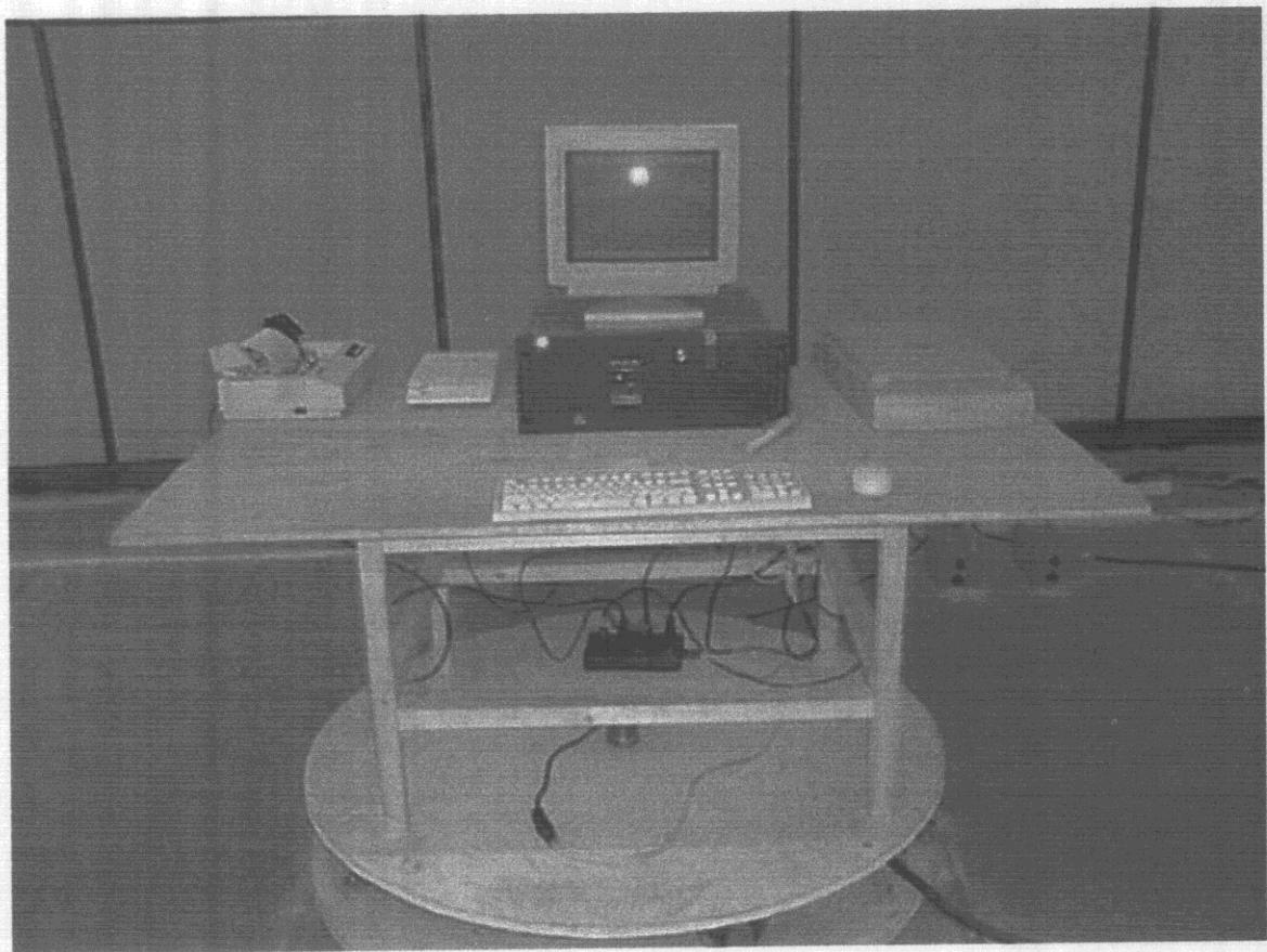
**6.4 Radiated Emission Photograph – Rear View**
