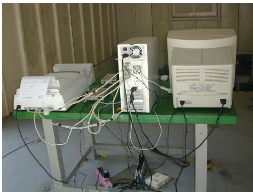
Back View of Radiated Test (Mode 2 —Link PC, W/1394 Cable (1.5M)
