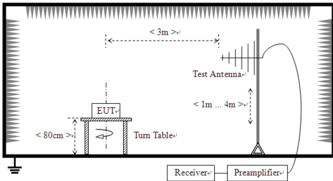
The EUT is located in a 3 m Semi-Anechoic Chamber; the antenna factors, cable loss and so on of the site as factors are calculated to correct the reading.
