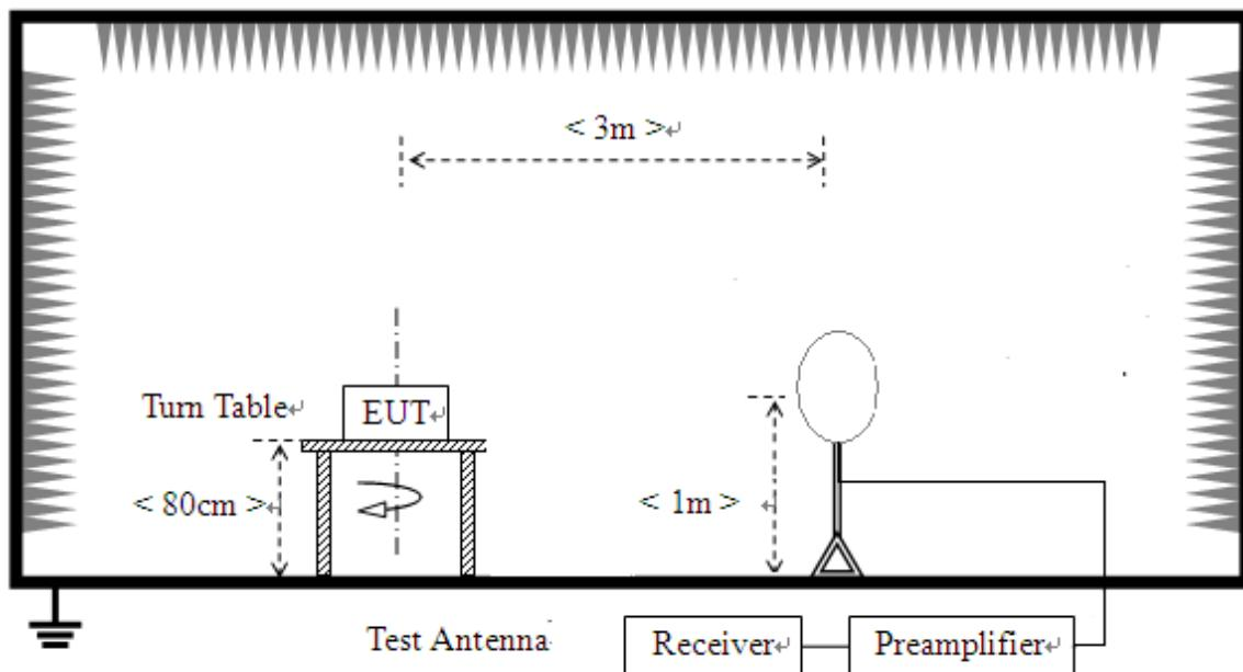
2) For radiated emissions from 30 MHz to 1 GHz
