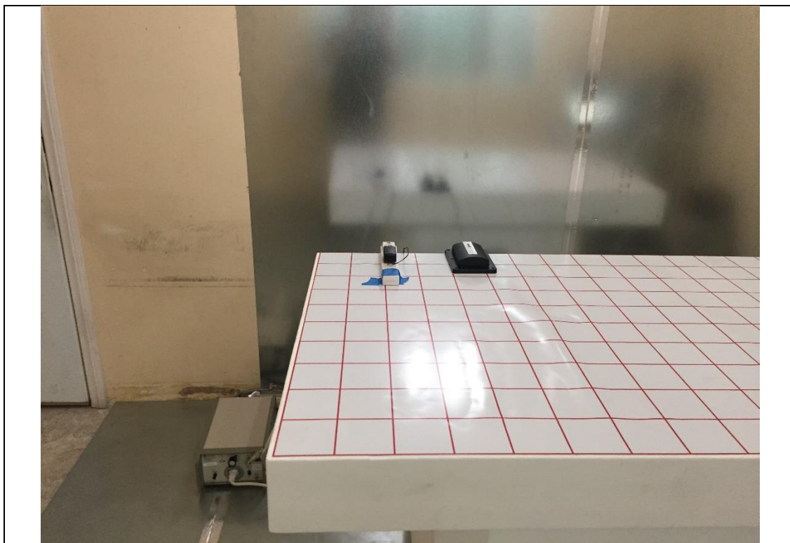
AC Line Conducted Emission setup – Front
