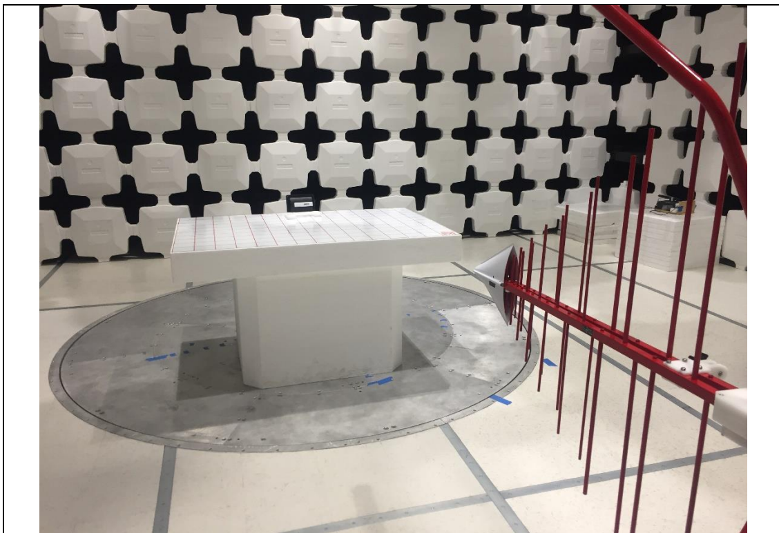
Radiated Emissions Below 1GHz setup – Front
