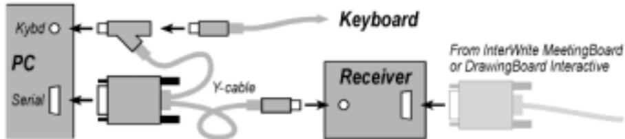
3. If your system includes an InterWrite MeetingBoard or DrawingBoard Interactive, connect it to the receiver with a 9-pin serial cable.
