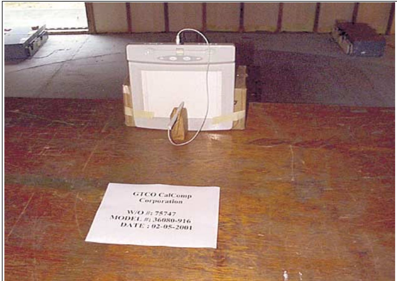
Radiated Emissions - Vertical Orthogonal
