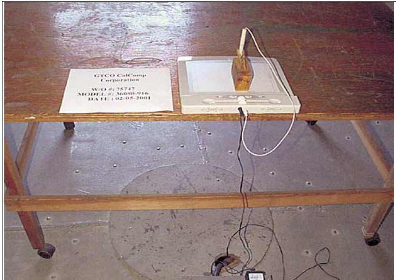
Radiated Emissions - Back View, Horizontal Orthogonal
