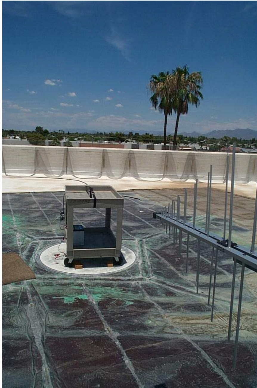
Figure C – 2 Radiated Spurious Emissions Test Setup, OATS
