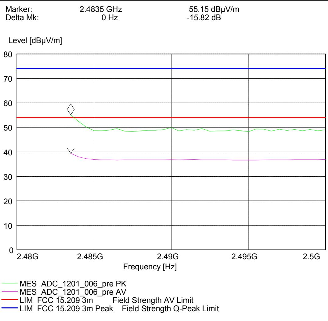
**Test: 15c.6; Frequency = 2480, Mode = BT transmit using 3 Mbps with 8DPSK modulation, Method = conducted**
