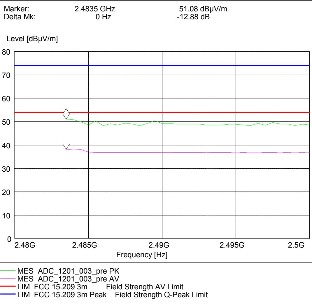
**Test: 15c.6; Frequency = 2480, Mode = BT transmit using 2 Mbps with PI/4 DQPSK modulation, Method = conducted**
