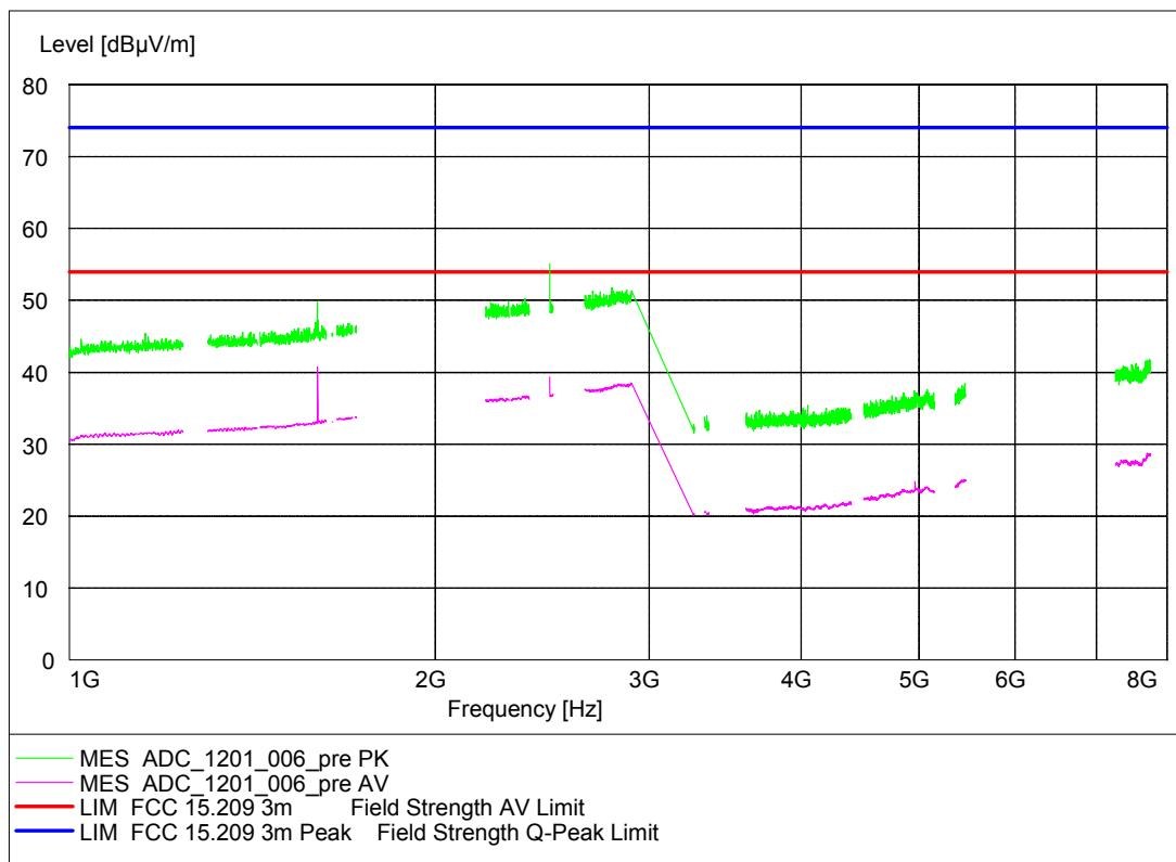
**Test: 15c.2; Frequency = 2480, Mode = BT transmit using 3 Mbps with 8DPSK modulation**
