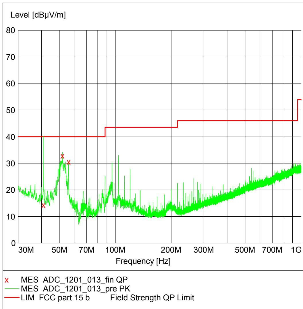
**MEASUREMENT RESULT: "ADC\_1201\_013\_fin QP"**
