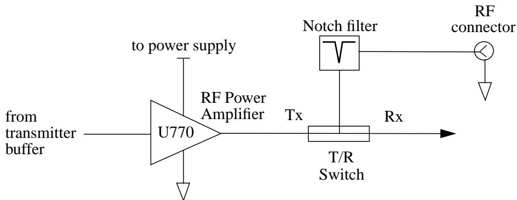
**CIRCUIT DESCRIPTION – MEANS FOR LIMITING POWER AT TWO WATTS****4. Means for Limiting Power at Two Watts**
