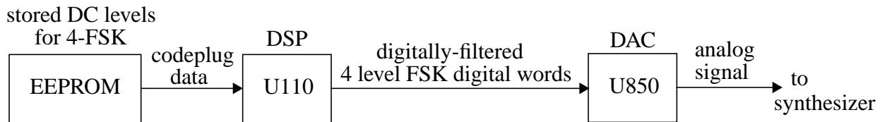
**CIRCUIT DESCRIPTION – MEANS FOR ATTENUATING SPURIOUS EMISSIONS****3. Means for Attenuating Spurious Emissions**
