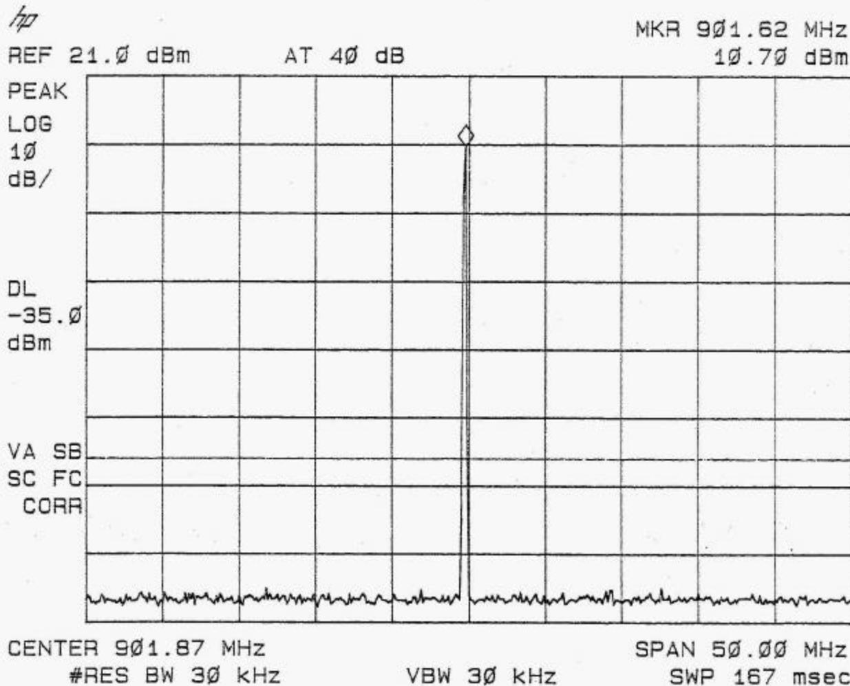
**SUBMITTED MEASURED DATA—SPURIOUS EMISSIONS AT ANTENNA TERMINAL**
