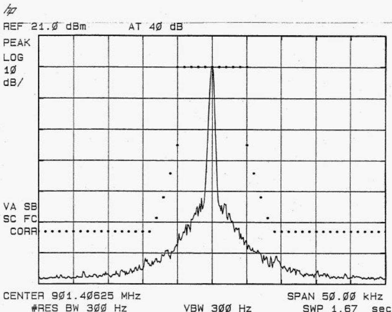
SUBMITTED MEASURED DATA - SPURIOUS EMISSIONS AT ANTENNA TERMINAL
