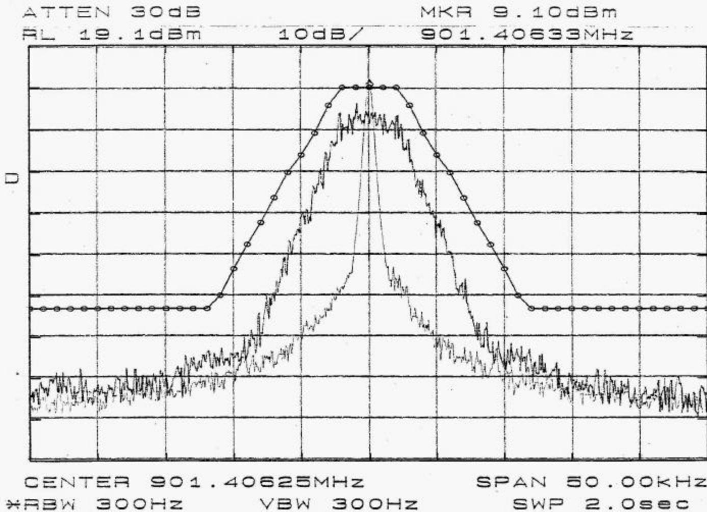
SUBMITTED MEASURED DATA- SPURIOUS EMISSIONS AT ANTENNA TERMINAL
