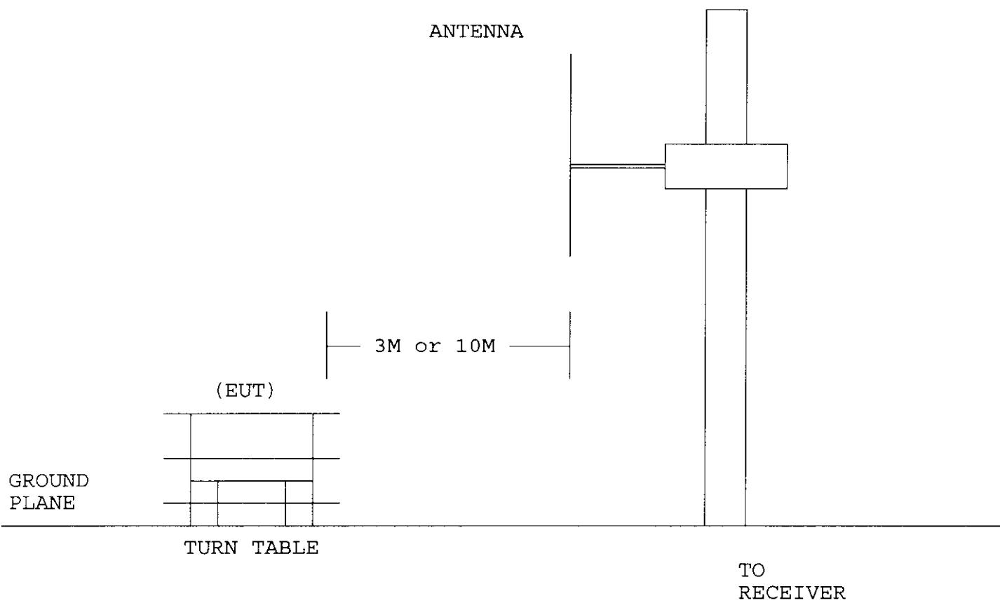
6.5 RADIATED TEST SETUP
