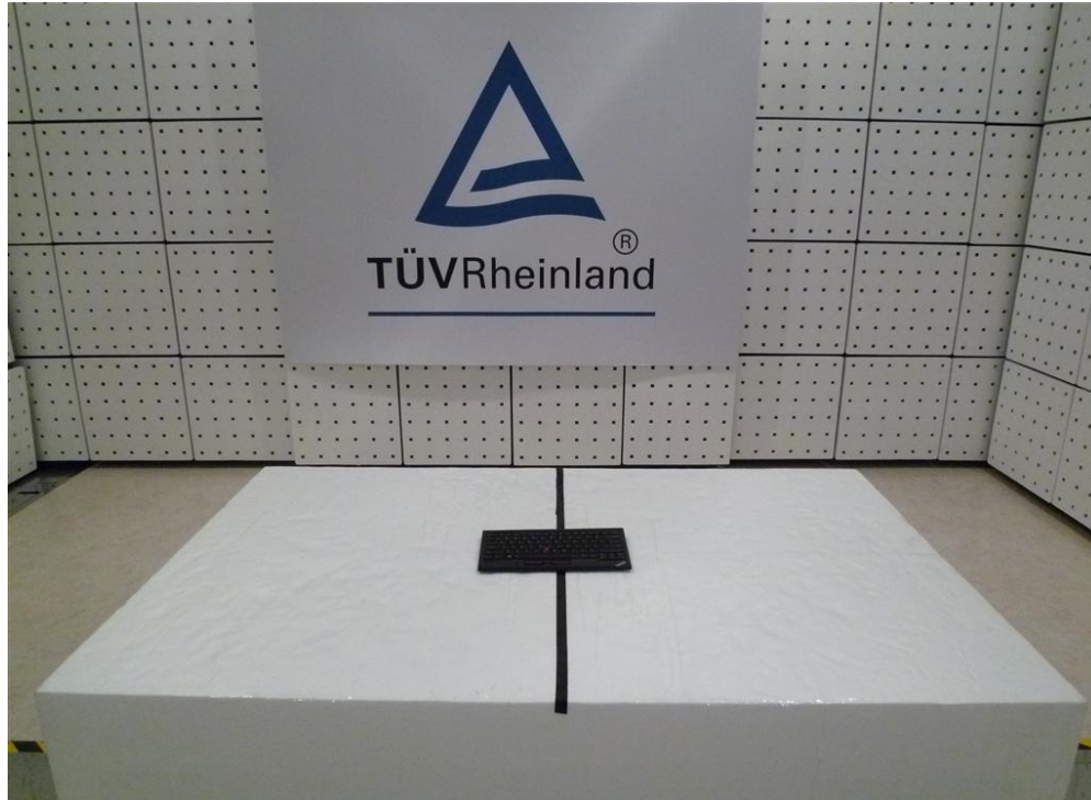
Photograph 2: Set-up for Spurious Emissions (Back View 1)
