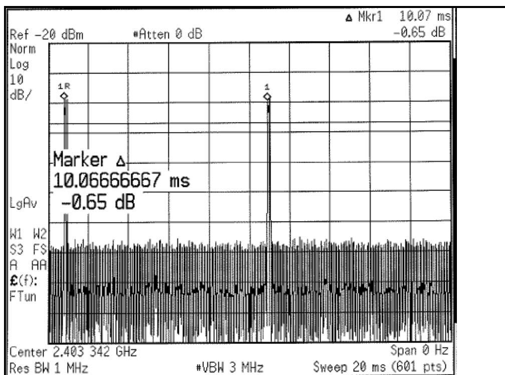
$$20 \log (\text{Duty cycle}) = 20 \log (0.133 \text{ ms} / 10.066 \text{ ms}) = -37.6 \text{ dB}$$
