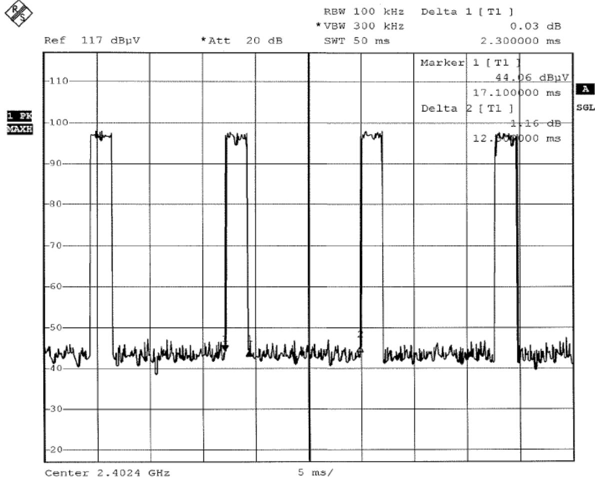
$$20\log(\text{Duty cycle}) = 20\log \frac{2.3 \text{ ms}}{12.8 \text{ ms}} = -14.9 \text{ dB}$$
